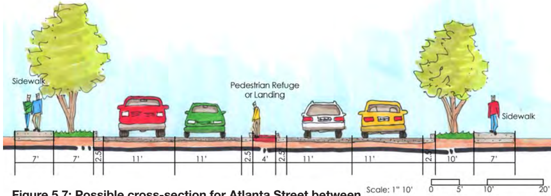
Figure 5.7: Possible cross-section for Atlanta Street between the Allenbrook and Barrington Roundabouts (Alternative 2)
